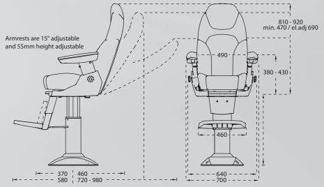
*Mounting holes measures - see page 31* - Working diameter of the chair folded Ø790. Expanded, with the backrest all the way down Ø1480. Weight 70 Kg.
