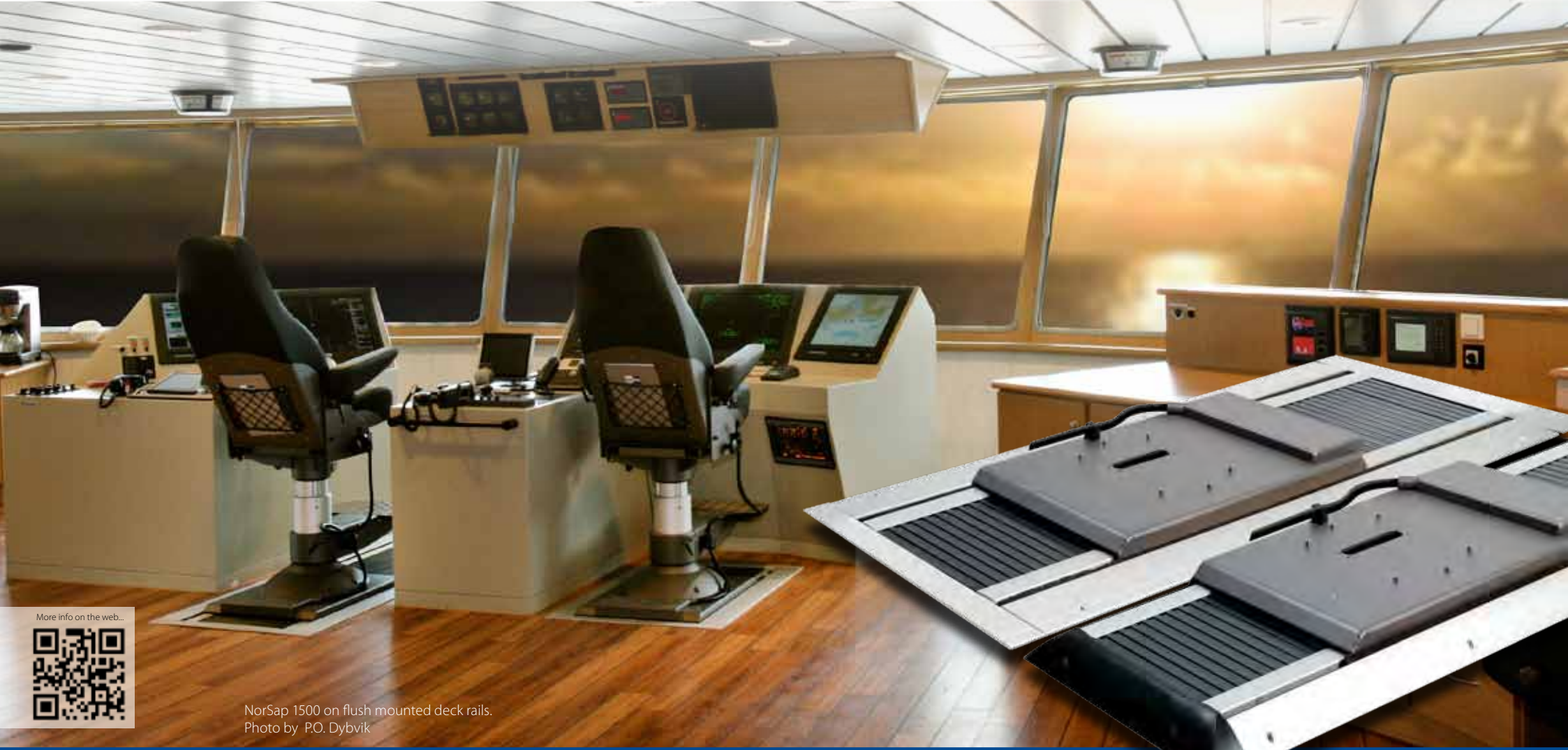
Flush and topmounted versions of the narrow deck rails.
